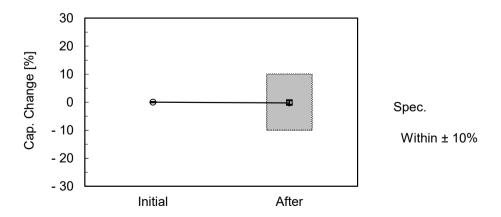
(Dielectric Strength) AC2600V(r.m.s.),60 s and DC3225V Dielectric Strength (Between lead wires) : No failure Dielectric Strength (Body Insulation) : No failure Insulation Resistance (I.R.) :  $1000M\Omega$  min.
